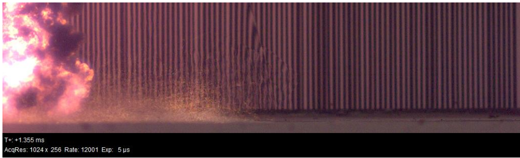
Figure 13. Hexomax ® blast wave propagation recorded with high speed camera ( t = 1.355 ms after charge detonation)
