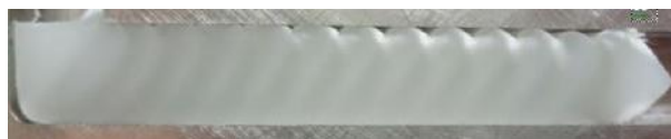
Figure 8. Macrographs of PP samples after a first pass ECAE at a ram speed of 45 mm/min.
