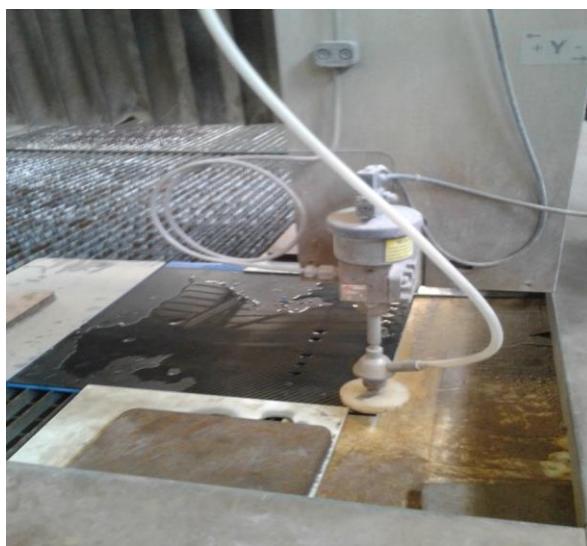
Figure 2. Water jet machine until machining CFRP plate
