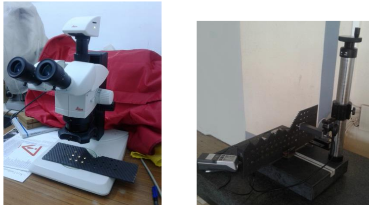
Figure 3. Instruments used in the experimental study: a) Microscope Leica M80, b) rugosimètre 2D mitutoyo SJ201P
