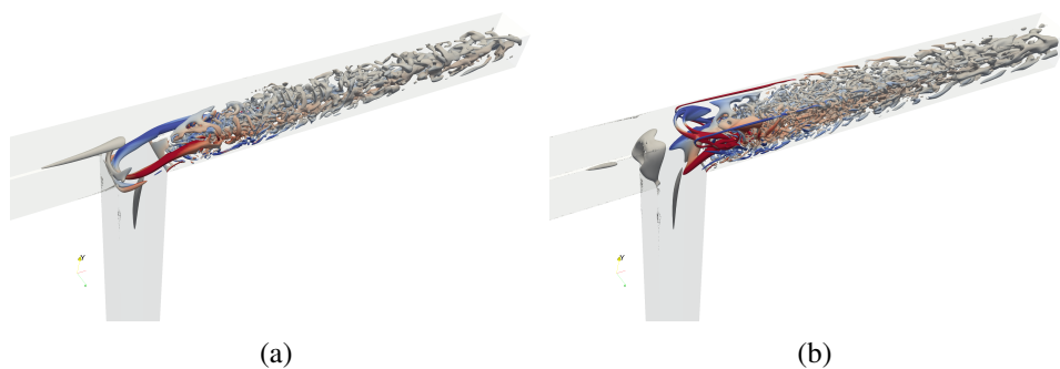
FIGURE 4 – Vortices visualization based on iso-surfaces Q^+ = 0.3 in a shear thinning T-junction flow : (a) Deflecting regime and (b) impinging regime. Red is plotted where vorticity's x-component is positive whereas as blue denotes the counter-rotating negative vortices.
