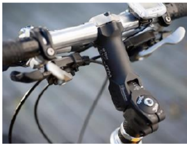
FIGURE 2 – Montage de potence A-Head-Set
