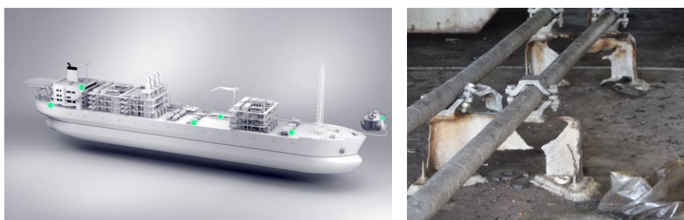
Figure 8: Corroded pipe support on top of FPSO Crude Oil tank
