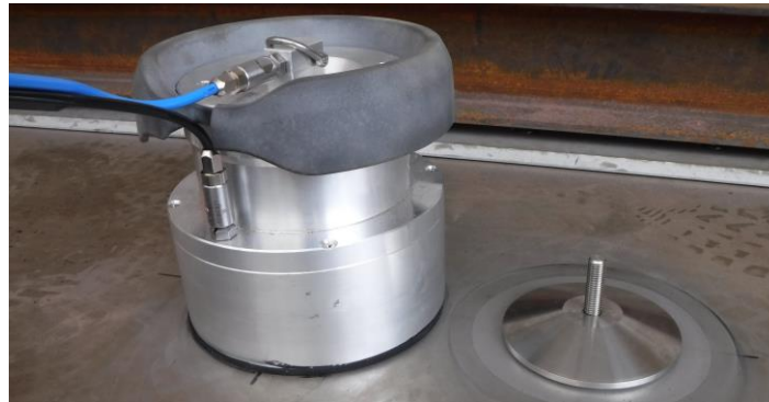
Figure 3: C-Claw TM (right) bonded on a steel plate with C-Hawk bell (left)
