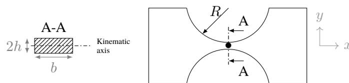
FIGURE 6 – Description of a flexible link and its minimum section
