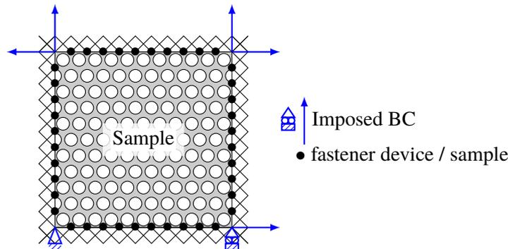
FIGURE 5 – Field application device by pantographic frame
