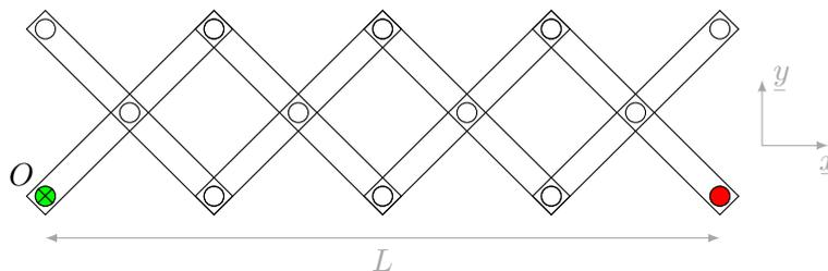
FIGURE 4 – Schematic diagram of a pantograph
