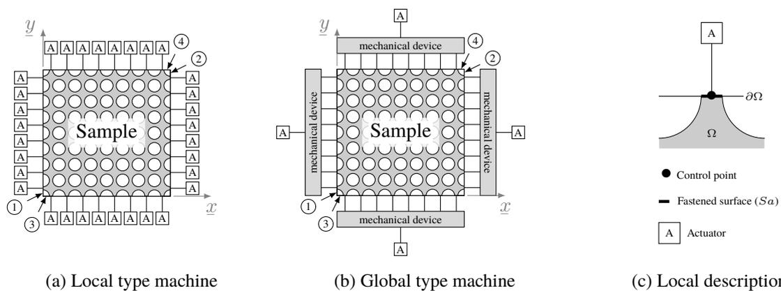
FIGURE 3 – Schematic diagram of local and global type devices
