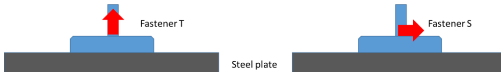
Fig. 5: Scheme of the two tested solicitation modes: Tension and Shear loadings.
