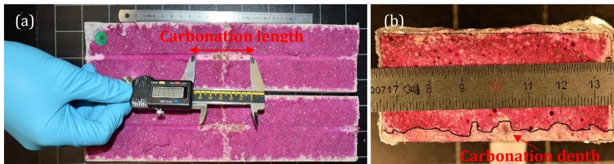
Figure 7 : (a) Carbonation length of the steel/mortar interface for cracked carbonated specimen; (b) Carbonation depth of uncracked specimen
