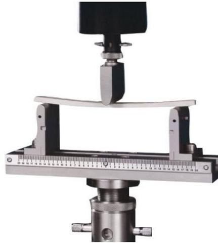
**Fig. 2.** The 3-point bending device.
