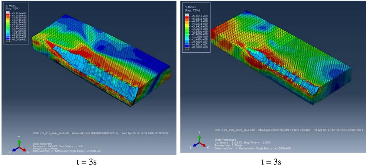
Figure 5: Von Mises stresses on sample with steel alone
