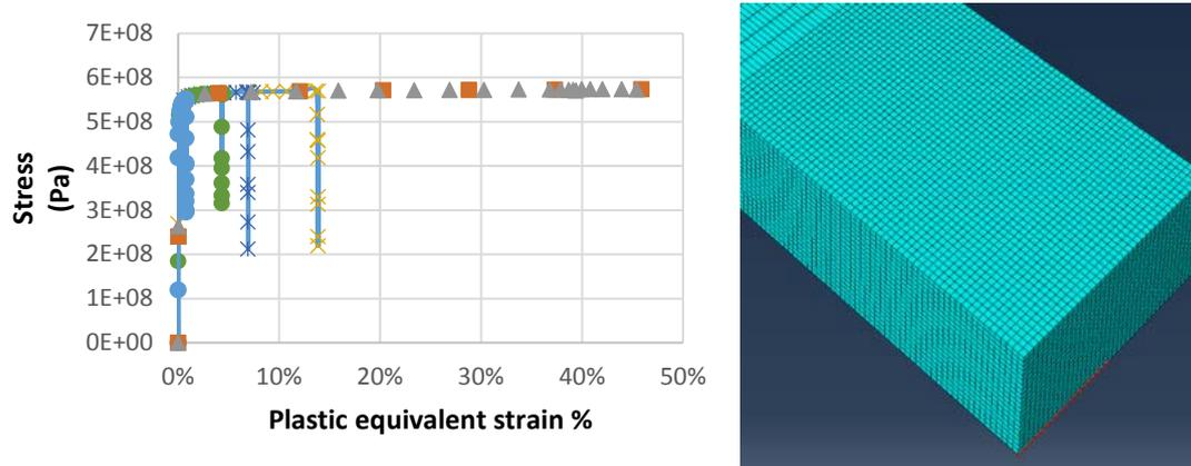
Figure 9: Evolution of the equivalent von Mises stress as a function of the equivalent plastic strain for different points of the line on the lower surface.
