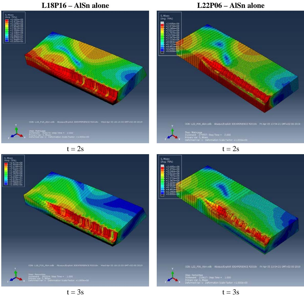
Figure 6: Von Mises stresses on sample with AlSn alone
