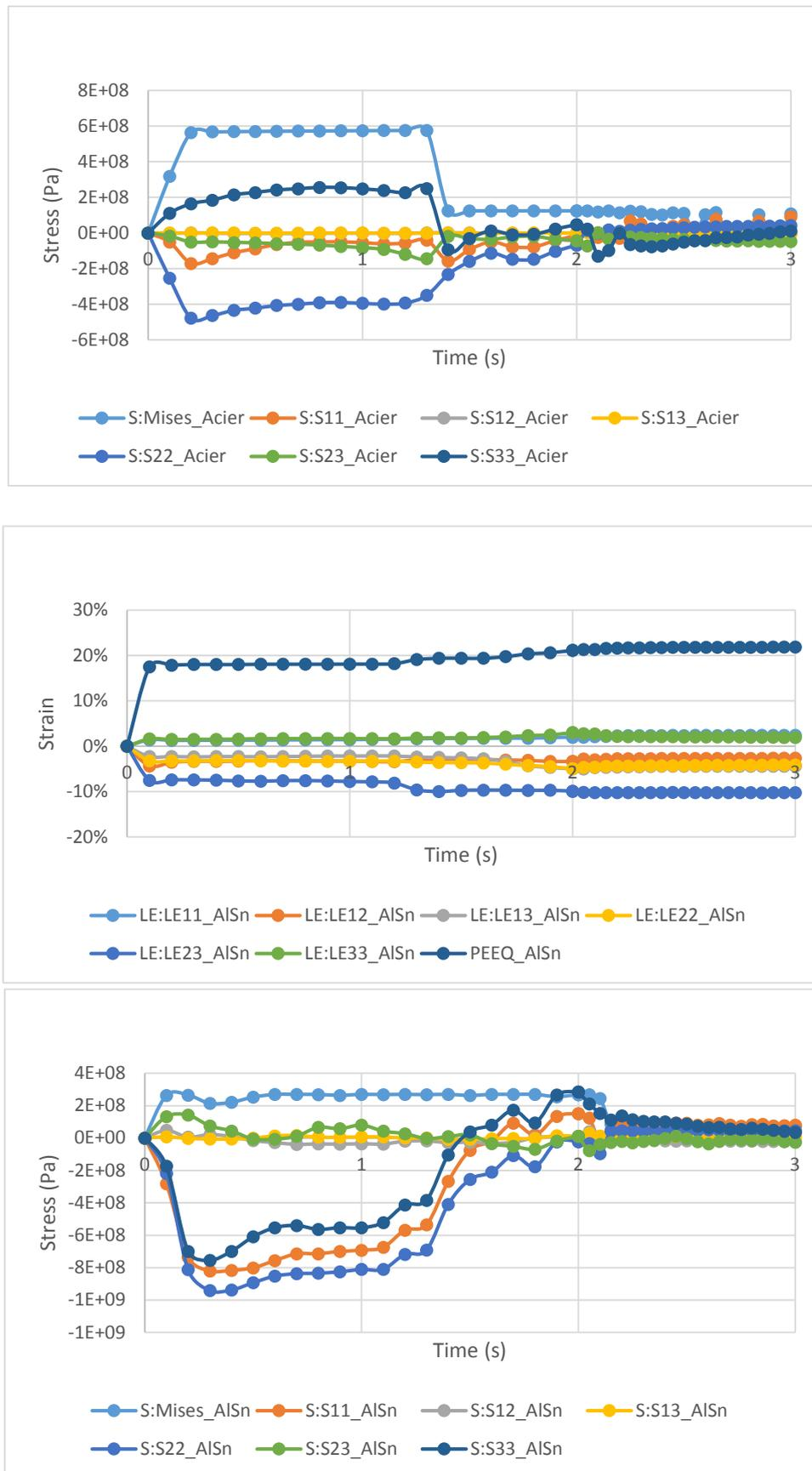
Figure 8: Temporal evolution of stresses and strains at the high and low center points of the sample during forming of bimaterial.
