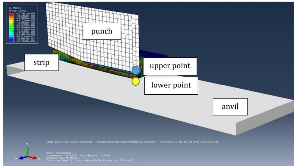
Figure 4: Numerical simulation of forming on sample L18P16
