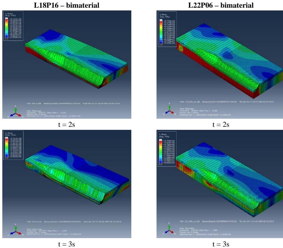
Figure 7: Von Mises stresses on sample with bimaterial
