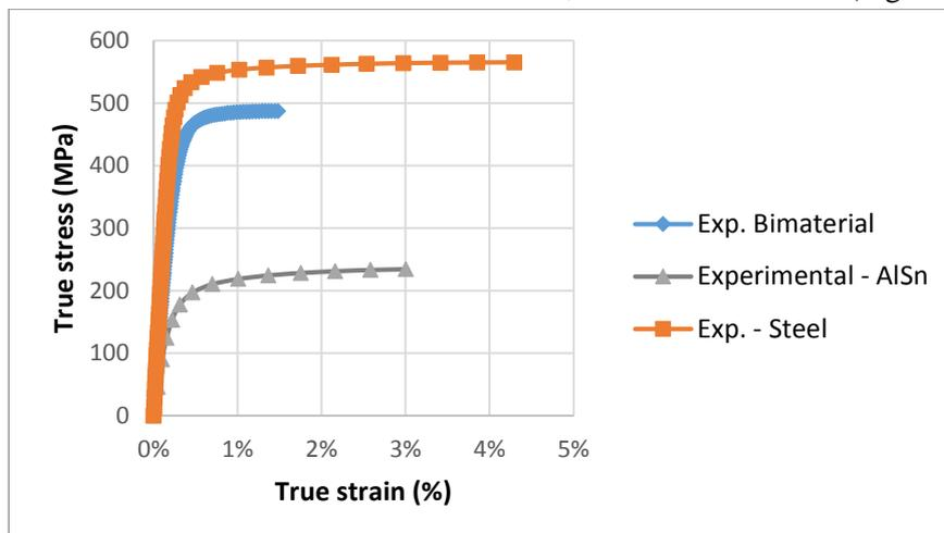
Figure 1: Tensile on steel, AlSn and bimaterial
