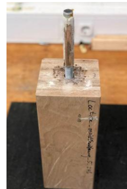
Figure 6: Failure pattern of a resistively heated probe with EP32, tested 24 h after curing
