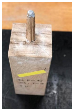
Figure 4: Failure pattern of an inductively heated probe with FIS EM, tested 24 h after curing
