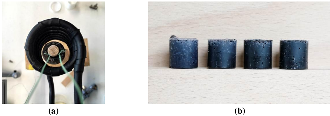
Figure 1: (a) Inductive heating of small cylindrical probes of adhesive-particle mixtures, temperatures were measured with two thermocouples; (b) Small cylindrical probes of adhesive-particle mixtures (height: 20 mm, diameter: 20 mm, thickness: 2mm)
