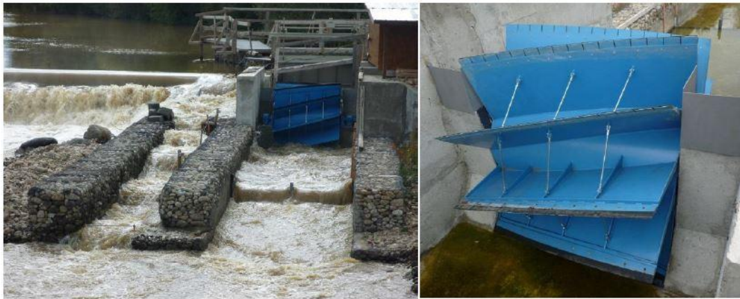
Figure 1. HPM under real field trial, developed by the HYLOW project, Bulgaria (pictures taken from [1]).
