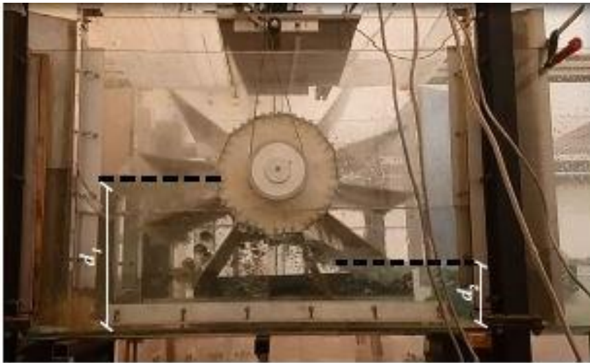
Figure 5. IRPHE HPM wheel operating in the Herode Channel. The water flows from the left and the wheel is rotating counterclockwise.
