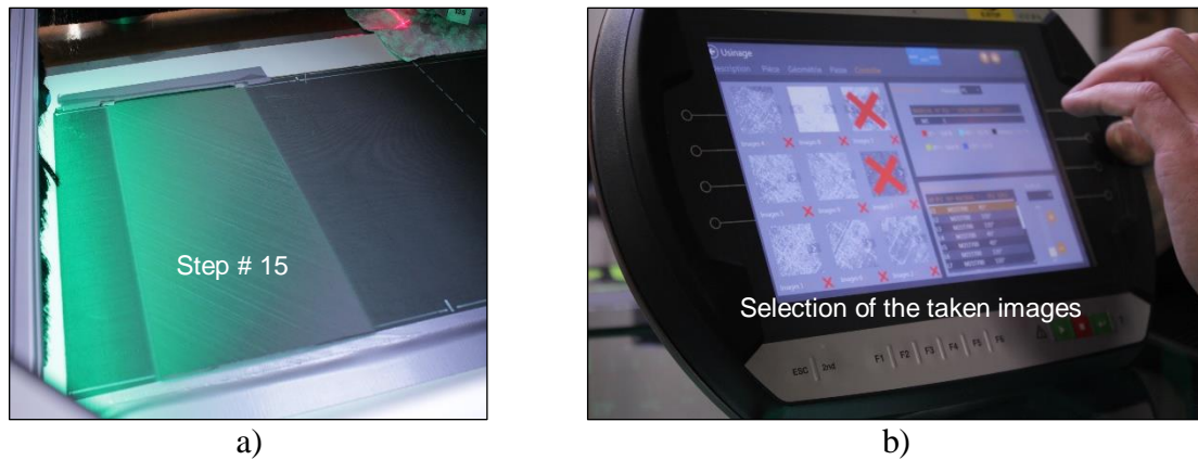
Figure 5. Verification process of the machining surface with a) overlap lap analysed by image analysis and b) visualization and selection of the taken images on the control panel to estimate whether or not the interface is reached.
