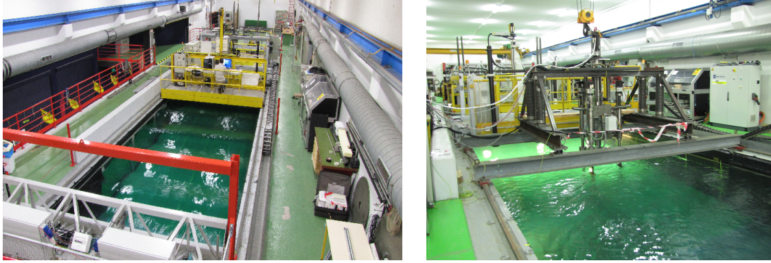
Figure 6 – Ifremer wave current flume tank overview
