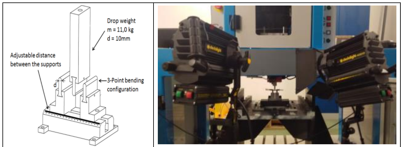
Fig . 6. Impact bending device on the drop test
