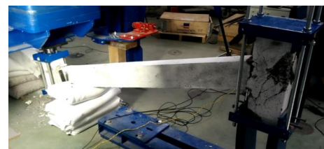
Fig. 4. Dynamic response of a beam-column subassembly under a middle column removal scenario
